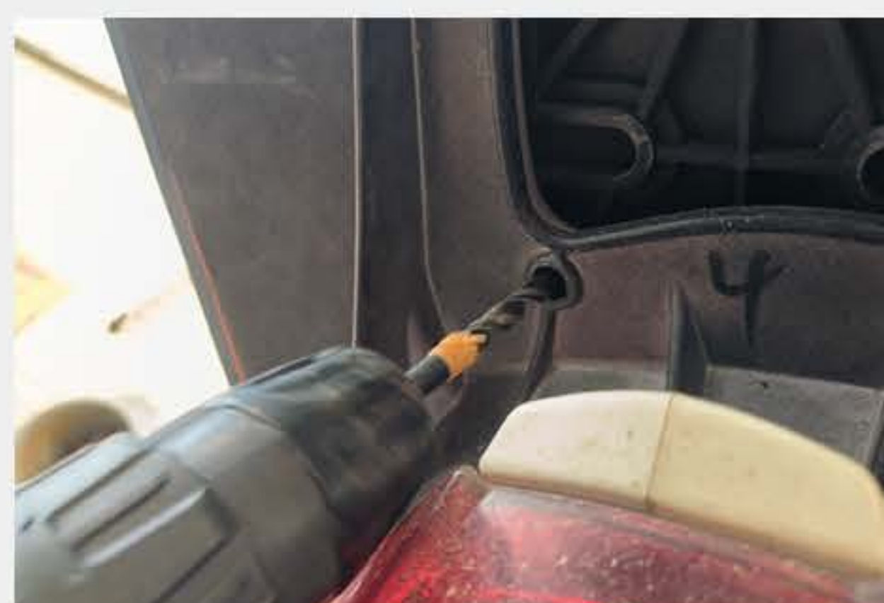
3. Drilling holes through the interior
