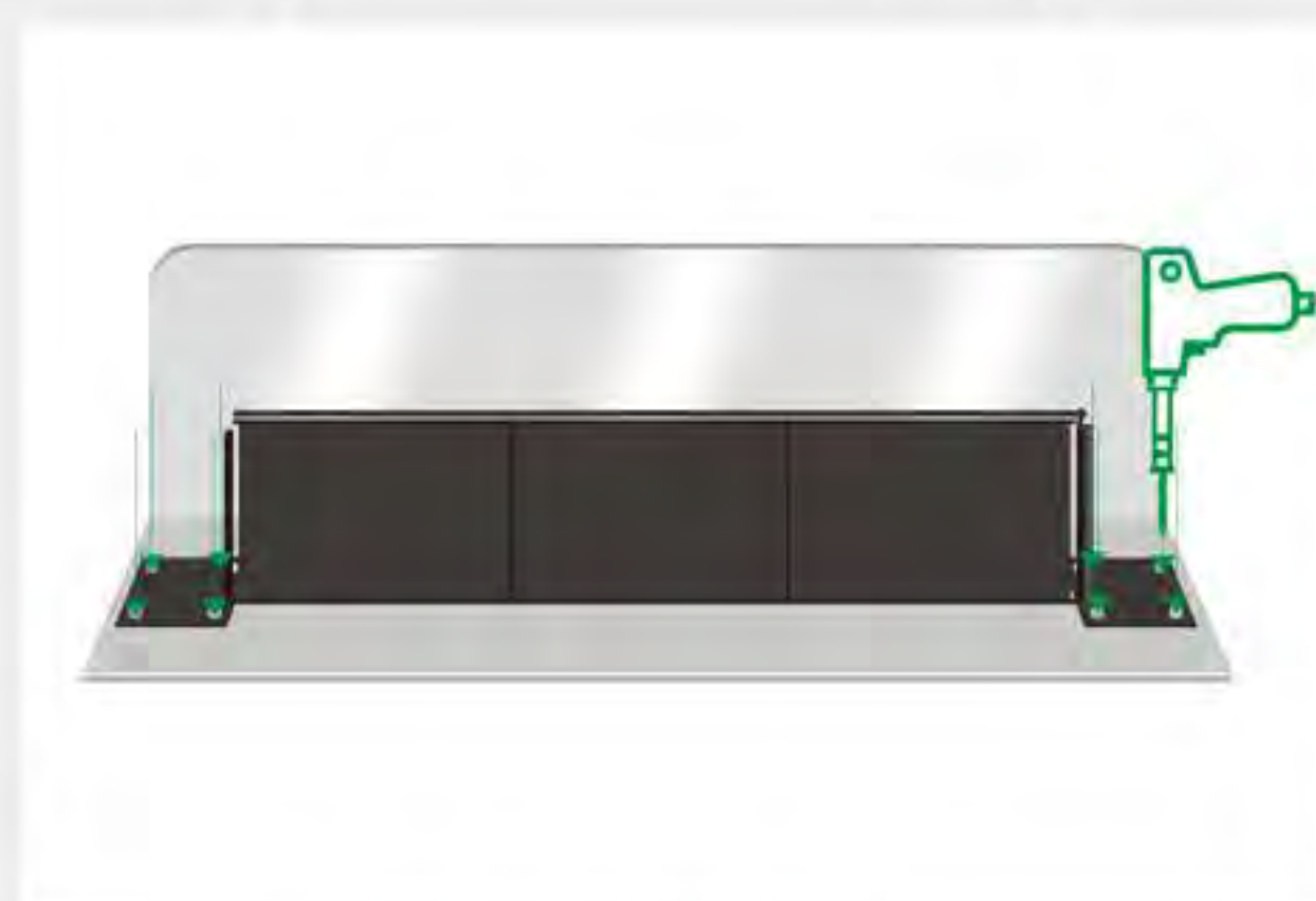
3. Drill wire holes
