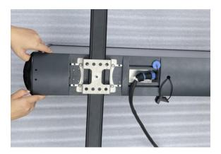
1. Align the white dot of the power cord with the white dot of the socket at the bottom of the double-sided screen.
