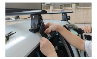
1. Paste the gasket underneath the hook of the luggage rack to prevent scratching the car body.
