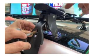
1. Pass the nut through the hook and tighten it against the nut inside.
