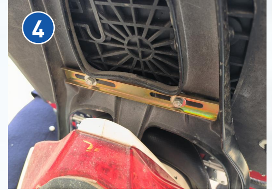
Install iron plate
