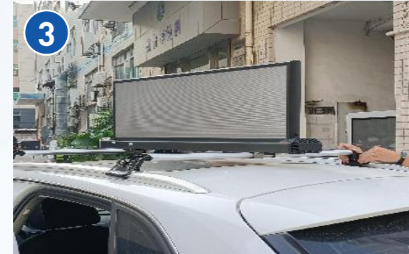
Put the double-sided screen on the roof of the car
