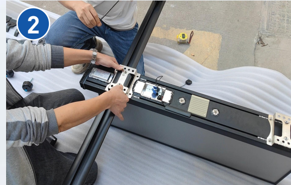
Lock the mounting bracket in On the bottom fastener
