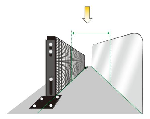
Keep a distance of at least 10CM between the bus screen and the rear window.
