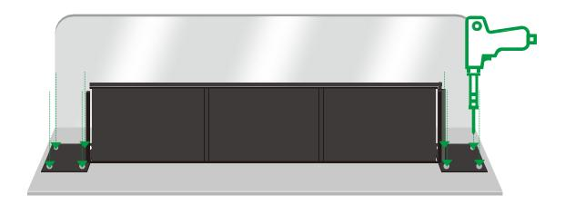
3. The power control compartment needs to be drilled. When drilling the base hole with an electric drill, it can be slightly larger than the diameter of the screw.
