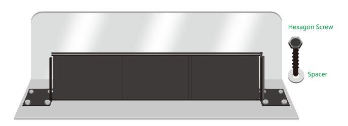
4. After the bracket is fixed on the base, Use 8 external hexagonal M8\*70mm screws and washers to fix.
